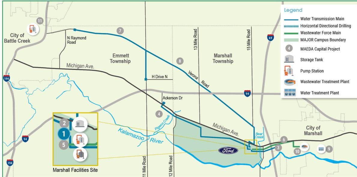
A High Service Pump Station (HSPS) will be constructed at the Marshall Facilities Site near Michigan Avenue and 15 Mile Road adjacent to Project #2, a 4.5-million-gallon (MG) Ground Storage Tank (GST). The HSPS will house four (4) pumps each rated at 1,800 gallons per minute (gpm) with a total station capacity of 10.5 million gallons per day (MGD).
