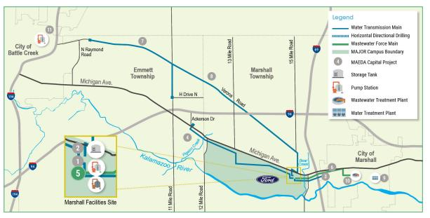
A Sanitary Pump Station (SPS) will be constructed at the Marshall Facilities Site located south of Michigan Avenue and west of 15 Mile Road. The SPS consists of a 12-foot diameter precast concrete wetwell with three (3) submersible pumps each rated at 800 gallons per minute (gpm). A standby power generator and remote monitoring telemetry are included.
