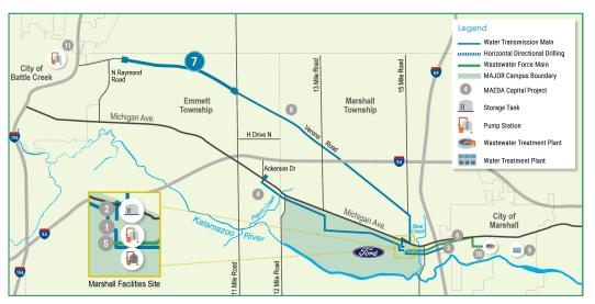
The Emmett Township Loop Water Transmission Main begins with a 20-inch diameter pipeline on Verona Road just east of Raymond Road. The main extends along Verona Road, making a connection with the Verona Loop Water Transmission Main (Project 8).
